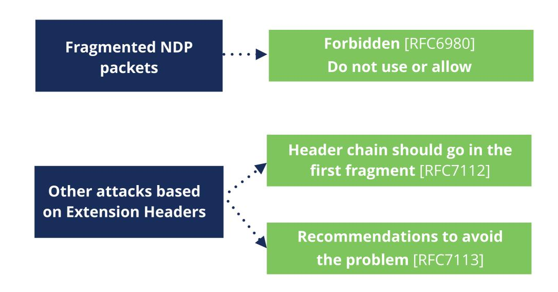
Require security tools to inspect Header Chain properly
