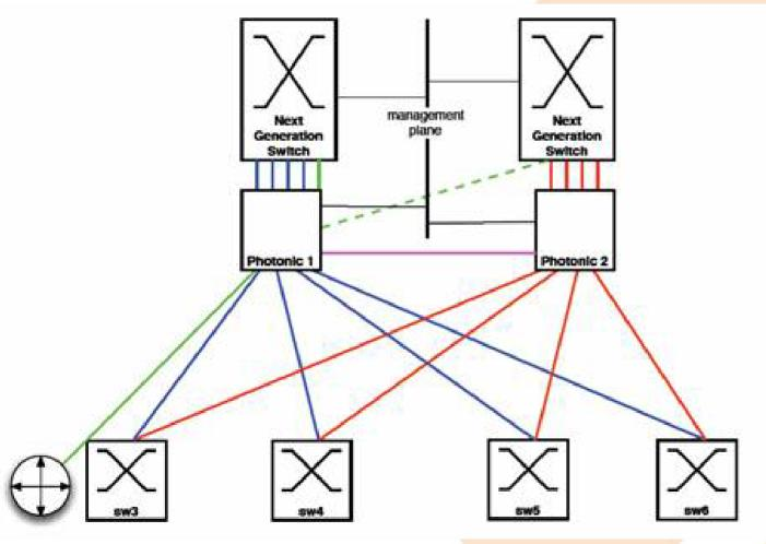
Upgraded infrastructure with fully redundant double star topology using photonic switching to build resilience and exclude any single point of failure
