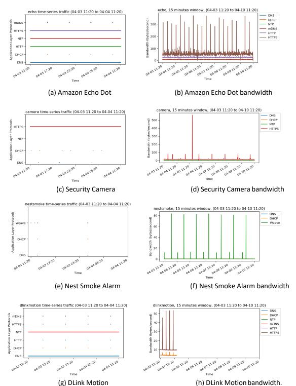
Figure 5: Time-series data representation of the traffic generated by each device, in terms of pattern in a 24h period and bandwidth (in 15 minute buckets) over a whole week.
