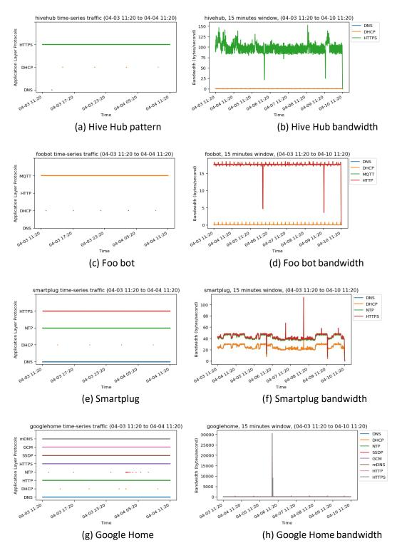
Figure 4: Time-series data representation of the traffic generated by each device, in terms of pattern in a 24h period and bandwidth (in 15 minute buckets) over a whole week.
