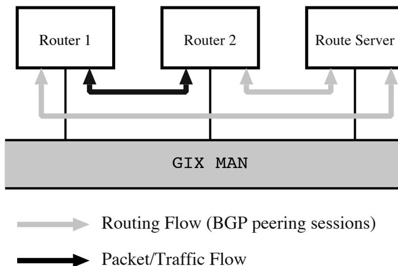
*Figure 1: General packet flow versus routing flow*
