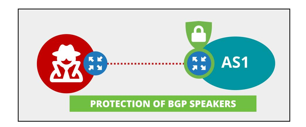
Only BGP peers to send packets to TCP 179: Control Plane Policing (CoPP), or ACLs (if CoPP not supported)
