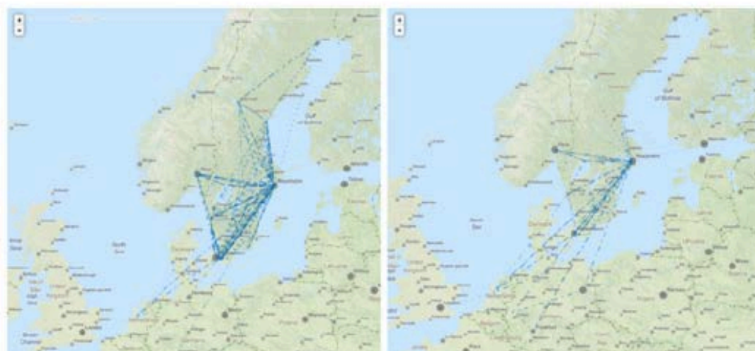
Figure 1: Visual representation of IPv4 paths (left) and IPv6 paths (right) between selected RIPE Atlas probes in Sweden
