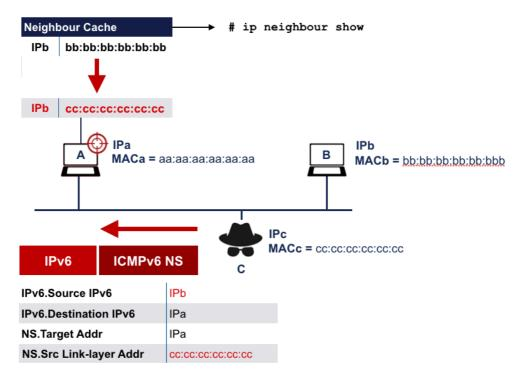
We will use Host C as the attacker, and two hosts that can be the target (A and B). All have an IP and MAC addresses, the ones shown in the scheme are just a reference, in this exercise use the **real IPv6 and MAC addresses**.
