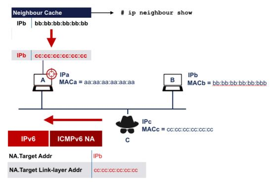
We will use Host C as the attacker, and two hosts that can be the target (A and B). All have an IP and MAC addresses, the ones shown in the scheme are just a reference, in this exercise use the **real IPv6 and MAC addresses**.
